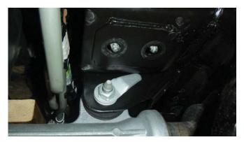
• Remove the manifold, studs out of the head they will not be used to install the header and remove the dip stick tube.
