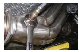
• Install the left front 02 sensor into the collector at this time and connect back into the wiring harness. Wire tie sensor away from any moving or hot parts using one of the supplied wire ties.
