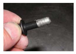
Install the two bottom rear headers bolts with the gasket on both sides. Only screw the bolts one two or three turns.
