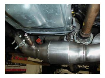
Install the left rear 02 sensor into the crossover pipe and plug it back into the harness and wire tie it up.
