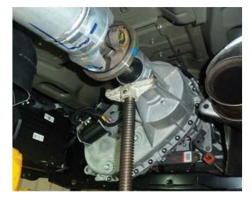
• Unbolt cats and remove the factory y-pipe and crossover as a unit.
