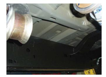
• Unbolt the heat shield from the top of the transmission cross-member on both sides. Right side picture shown.
