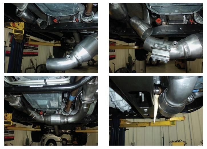
• Grind the locating pin on the end of the tube of the muffler off to allow the use of the supplied band clamp as the connection of the extension tube and muffler. After the pin is removed slide the band clamp over the end before installing the extension tube.
