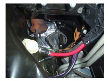
Note: The removal of the right side manifold will require raising the engine. The left side will come out without having the engine raised. You can remove both sides with the engine raised or remove the left side with the engine down and then raise the engine to remove the right side. The following steps for the left side will be with the engine down.
