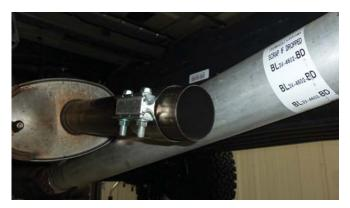
• Move the muffler back in its hanger far enough to install the extension tube but do not allow the mounts for the tailpipes to come out its hanger so it will stay in held up in place while installing the extension tube.
